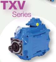
Variable displacement pumps with flow and pressure regulation (Load Sensing), perfectly suited to truck hydraulics, extremely compact in size . Displacement from 40 to 150 cc/rev.
